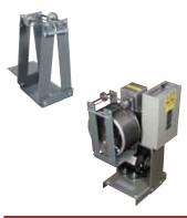
for draw curtain machines equipped with 5" x 10" drums or 7" x 10" drums
