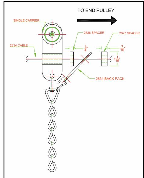
**Note:** Do not use back-pack guides on master carriers or the last single carrier of any system.
